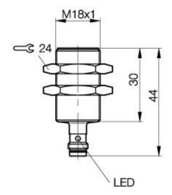
Inductive Sensors BES 516-355-G-E5-Y-S 49 M18x1 x 44 normally-open Sn=8mm shielded
